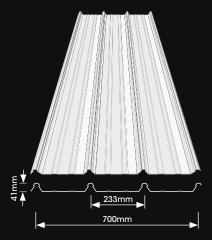
Cover width: 700mm Total width: 750mm Coil width: 925mm All dimensions given are nominal
